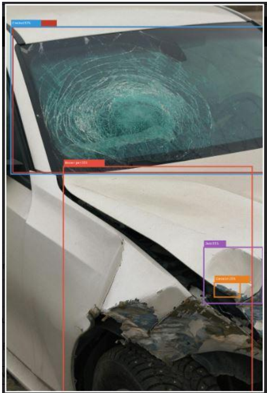
Figure 8. Sample annotated output from the AI inspection system showing detected damage with bounding boxes, class labels, and confidence scores.
