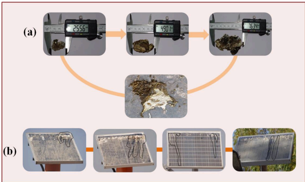
Figure 2: Effect of partial shading caused by bird dropping on a photovoltaic module.
