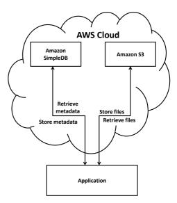
Figure 3: Data storage in the AWS cloud using S3 and SimpleDB
