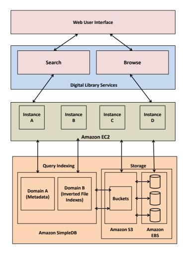
Figure 2: Conceptual design showing high-level system architecture
