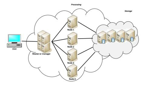
Figure 1: The Proxy Architecture: The "Master" or "manager" acts as a proxy between users and the cloud nodes
