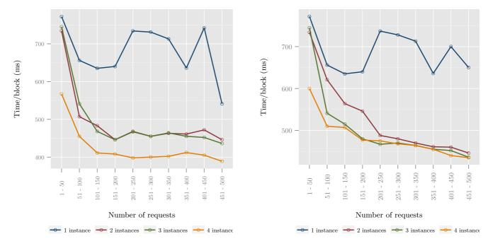
Figure 9: Plot of time in milliseconds (ms) vs. number of requests when searching the collection over a varying number of EC2 instances
